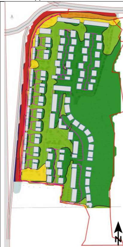
Figure 3: Revised Assessment - Lday road traffic noise contour bands with 10-year traffic increase.
